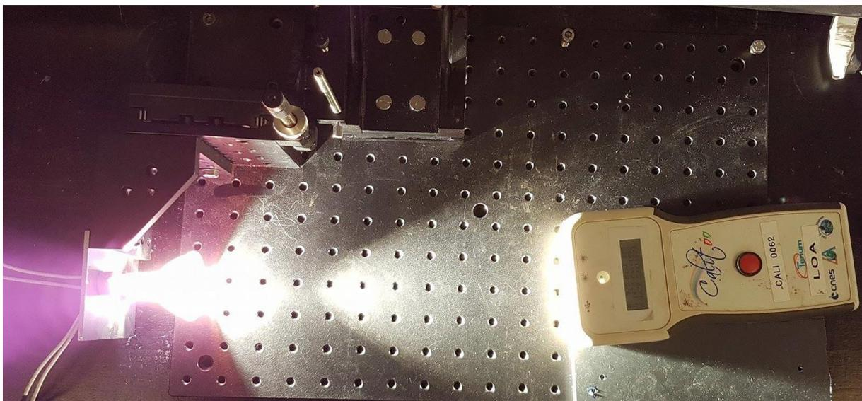
Optical bench used for the calibration
