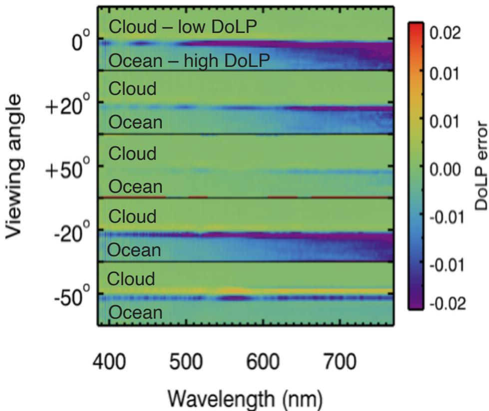
**For most challenging case factor 10 correction is needed. For the vast majority a factor 5 is sufficient.**
