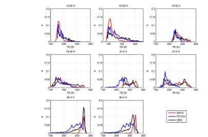
Fig-8. Normalized histograms of observed and simulated TBs (by ARTS and RTTOV-SCATT) in selected TMI channels.
