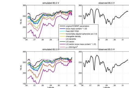
Fig-4. The observed and simulated brightness temperatures under different microphysical properties of snow at 85.5 GHz for the transect of interest.
