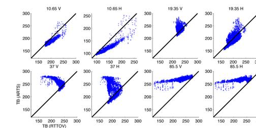
Fig-6. TBs simulated by RTTOV-SCATT against the TBs simulated by ARTS at TMI frequencies turning on the cloud box.
