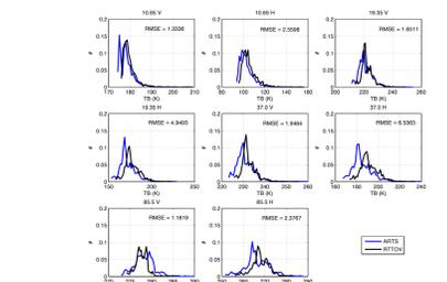
Fig-7. Normalized histograms of the simulated TBs by ARTS and RTTOV-SCATT in selected TMI channels for Irene case without considering the cloud cover.
